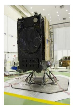
Galileo dispenser testing using the QUAD electrodynamic shaker during December 2010. The tests are using a qualification model of the dispenser, along with the with a pair of engineering models of Galileo IOV satellites, respectively the Structural Model (SM) and Structural and Thermal Model (STM). Credit: ESA
