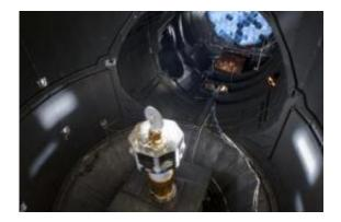
This is BepiColombo's Mercury Magnetospheric Orbiter (MMO) in the Large Space Simulator at ESTEC, the Netherlands. The octagonal spacecraft is Japan's contribution to BepiColombo and will explore Mercury's magnetic field. Credit: ESA/JAXA
