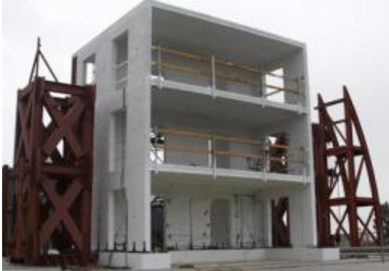
This three-story masonry structure with shear wall systems will undergo a series of severe simulated earthquakes at the UC San Diego Englekirk Structural Engineering Center, home of the world's largest outdoor shake table.
