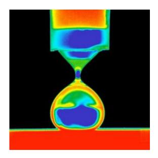
This image from a high-speed camera shows a droplet being deposited on a superhydrophobic surface, just before it separates from the dropper used to deposit it. At the moment of separation, ripples move down through the droplet, revealing the sudden deceleration caused by impact with the surface, which causes a brief burst of high pressure. Credit: Kripa Varanasi
