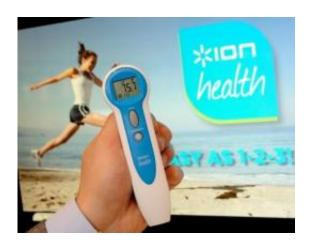
The USB Insta-scan Thermometer from Ion Health is displayed at the 2011 International Consumer Electronics Show at the Las Vegas Convention Center in Las Vegas, Nevada. The USD 90 device can acquire non-contact temperature readings from 1.2 inches away from the skin and upload data via USB 2.0 to a computer where it can be used with Ion Health Suite software.
