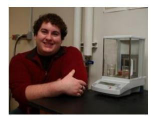
Patrick Bowen tracks the weight gain of a brick sample, part of his research to refine a new technique for dating old ceramics.
