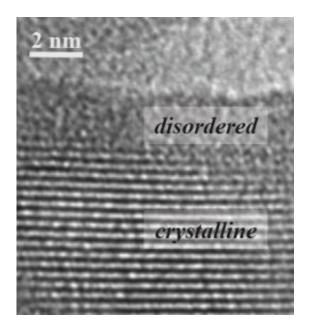
A nanoscale look at a photocatalyst that is both durable and very efficient. This high-resolution transmission electron microscope image of a titanium dioxide nanocrystal after hydrogenation reveals engineered disorder on the crystal's surface, a change that enables the photocatalyst to absorb infrared light.
