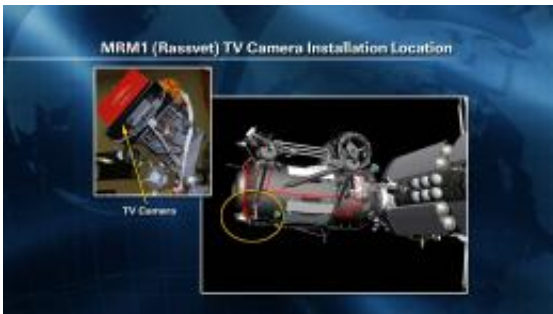
The MRM1 (Rassvet) TV camera installation location. Credit: NASA
