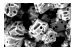
A magnified view of microbially generated calcite crystals reveals pill-shaped impressions left by the microbes.
