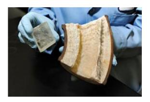
Bacteria and hard water can give heavy metals a hard time. Scientists coax underground microbes to turn calcium-rich water and urea into a stony underground trap for contaminants.
