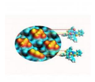
A scanning tunneling microscopy image (left) shows four porphyrins. The models (right) illustrate the two systems shown in the picture. The protrusions correspond to the central atom (yellow sphere) and the two elevated portions to the saddle (orange). The characteristic cross shape results from the attached carbon monoxide molecules (red and blue). Credit: Knud Seifert (TUM)
