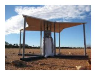
Close up of the EDGES antenna. The four panels are made from aluminum sheet metal and supported by PVC legs. The white bag under the antenna encloses analog amplifiers and calibration circuits. Credit: Judd Bowman/Arizona State University
