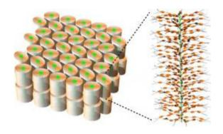
The light-responsive film is made up of polymer brushes (right) that have self-assembled into a two-layer, three-dimensional array (left). Credit: Reproduced, with permission, from Ref. 1 2011 American Association for the Advancement of Science
