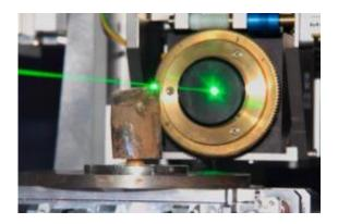
Fragment of the habitation chamber of a *Baculites* fossil (AMNH 55901), mounted on the mictotomography beamline ID19 at the ESRF. The laser symbolizes the position of the X-ray beam which first traverses the fossil and then hits the detector. Credit: ESRF/I. Montero
