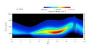
Contour plot of the electron density as a function of magnetic local time (MLT) and altitude. A fully 3D spatial model of ESF describing the motion of ions along and transverse to the geomagnetic field in a narrow longitudinal wedge of the post-sunset ionosphere. Credit: U.S. Naval Research Laboratory (2010)
