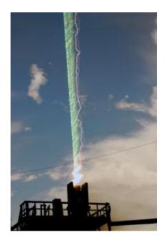
Rocket-triggered lightning allows scientists to measure the properties of a bolt. Credit: Dustin Hill / International Center for Lightning Research and Testing
