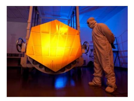
The James Webb Space Telescope's Engineering Design Unit (EDU) primary mirror segment, coated with gold by Quantum Coating Incorporated. The actuator is located behind the mirror. Credit: Photo by Drew Noel
