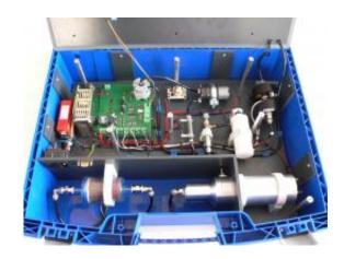
Chimney sweeps and heating engineers can use the portable measuring equipment to determine particulate concentration in a stove. Credit: Fraunhofer ITEM
