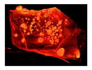
Silicate material mixed with iron shown at low pressure, with iron forming small, discrete spheres (lighter-colored areas) inside the silicate. Illustration courtesy of Wendy Mao
