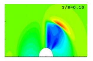
Model results of the water speed around a turbine blade. Currents are slower (blue) behind the blade, and faster (red) at the blade's tip. Credit: University of Washington
