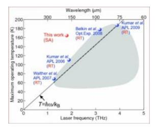
Terahertz lasers built in the lab had previously had operating temperatures (grey region) whose maximum values suggested a linear correlation with frequency. The new laser's operating temperature (red sphere) is nearly twice as high as that correlation would suggest. Graphic courtesy of Qing Hu
