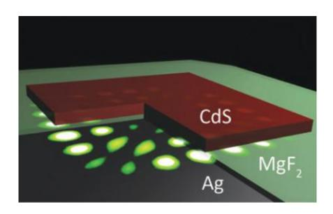
Schematic of a plasmon laser showing a cadmium sulfide (CdS) square atop a silver (Ag) substrate separated by a 5 nanometer gap of magnesium fluoride (MgF2). The cadmium sulfide square measures 45 nanometers thick and 1 micrometer long. The most intense electric fields of the device reside in the magnesium fluorid gap. (Renmin Ma and Rupert Oulton)
