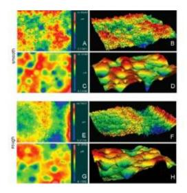
These images show the surface profiles of the adhesive side of peeled tape, obtained with the use of a white-light interferometer. A-D show a smooth surface due to fast peeling, while E-H show a rough surface due to slow peeling. A, B, E, and F are at low magnification, while C, D, G, and H are at high magnification. Image credit: B. N. J. Persson, et al.
