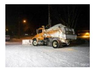
A snow plow and road salt application truck is used to clear snow and ice from roadways. Credit: Steven Corsi, USGS
