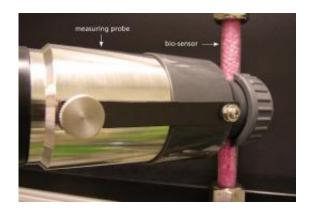
The red fluorescent bacteria in the glass tube change their color whenever the microorganisms in the bio-sensor come into contact with toxic substances. The measuring probe shows the intensity of fluorescence. Credit: Fraunhofer IGB
