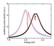
Scattering spectra for the structure when the corners of the metal nanoparticles have a curvature of 5 nm (solid squares) and 2 nm (open squares), calculated using the FDTD method. The lines are fits to a coupled-oscillator model.
