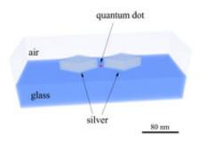
A quantum-dot/metal nanoparticle hybrid structure that could be fabricated lithographically.
