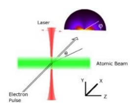
A color JPEG image of a figure that illustrates an experiment modeled by Hua-Chieh Shao and Anthony Starace. It shows the 110-attosecond electron pulse sent through a beam of hydrogen atoms (green) excited by a laser (red).
