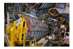
An engineer on a headset helps guide a space shuttle main engine into space shuttle Atlantis. The decision to have someone on top of the engine installer came about by accident during the first engine installation on Columbia 30 years ago. Photo credit: NASA/Kim Shiflett
