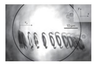
Time-lapsed composite image (1.67 s per shot) of a semi-cylindrical rod lifting sideways from left to right near the bottom of a glass chamber, as a result of a transverse optical lift force. Image credit: *Nature Photonics*, doi:10.1038/nphoton.2010.266
