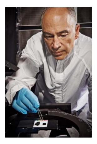
Principal Investigator John Hagopian developed a new nanotech-based material that is 10 times more effective than black paint used by instrument developers to absorb stray light, which can contaminate scientific data. The sample on the left is black paint typically used to suppress errant light in instruments; the sample on the right is the new nanotube material. Credit: Chris Gunn/NASA
