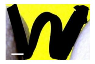
Flexible carbon nanotube material. Scale bar is 1mm. Image credi: Science, DOI:10.1126/science.1194865
