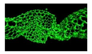
High-intensity atomic-level sonic boomlets cause nanotubes to buckle and twist at "compression-concentration zones." Credit: Kyung-Suk Kim Laboratory, Brown University
