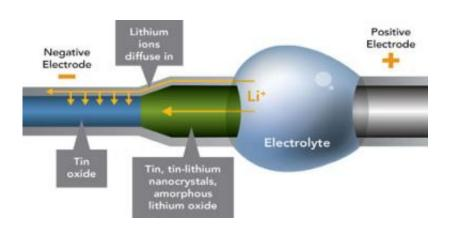
This nano-sized battery reveals how positive lithium ions flood the negative electrode (blue), changing the size, shape and nature of the material (the green part of the electrode). Some rechargeable materials might be more resilient than others to the repeated shape-changing.
