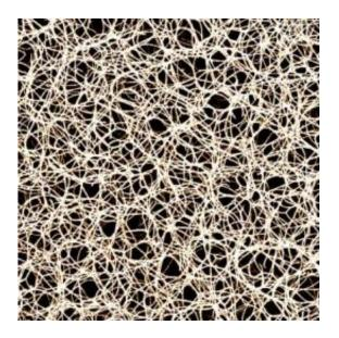
With the aid of a confocal rheometer, researchers can test the mechanical properties of a polymer network and, at the same time, capture images of the microscopic structure. Credit: Copyright TU Muenchen, all rights reserved.
