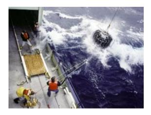
A CTD (conductivity, temperature and depth) sensor system is lowered into the ocean in preparation for recording the kinds of measurements that can now be predicted using a system developed by MIT's Pierre Lermusiaux and his colleagues. Photo: Woods Hole Oceanographic Institution
