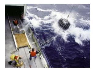
A CTD (conductivity, temperature and depth) sensor system is lowered into the ocean in preparation for recording the kinds of measurements that can now be predicted using a system developed by MIT's Pierre Lermusiaux and his colleagues. Photo: Woods Hole Oceanographic Institution
