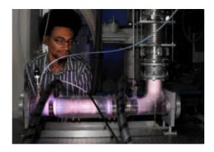
PhD student Gilles Adande monitors the reaction chamber in which the methanemetal hybrid molecule is produced. Ionized gas inside the chamber emits a pink glow.
