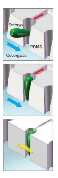
These schematic diagrams show the embryo trapping process: (top) the crossflow guides an embryo into the cylindrical trap; (middle) the flow around the embryo orients it vertically; (bottom) the trap contracts after loading is finished and secures the embryo inside the trap. The yellow plane represents the focal plane where images are obtained. Credit: Georgia Tech/Hang Lu
