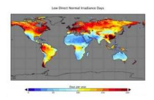
The average number of days per year when thermal CSP power plants cannot operate due to low direct normal irradiance levels. During many of these days, these plants are expected to still produce power using a backup system using natural gas or biomass. This feature allows CSP plants to produce reliable power year-round. Reprinted from Energy Policy, Vol 38, Author(s), Zhang, Y., SJ Smith, GP Kyle, and PW Stackhouse Jr., Pages 7884-7897, Copyright 2010, with permission from Elsevier.
