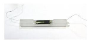
The apparatus shown here contains a phosphorus-doped silicon chip, only 1 millimeter square, that was used to demonstrate how data can be stored in magnetic "spins" within the centers or nuclei of phosphorus atoms, and then how that data can be accessed and read electronically. Credit: C. Dane McCamey, University of Utah.
