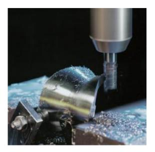
Intelligent software from Siemens for virtual planning and for the control of machine tools is making it possible for medical implants to be manufactured faster and less expensively. The challenge with artificial knee, shoulder, or hip joints lies in the fact that the materials, such as titanium or chromium cobalt, are very difficult to machine, but the complex shapes must be produced very precisely in order to provide an optimal fit for the patient.
