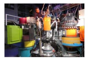
Looking for magnetic interactions: A technician adjusts the spectrometer which a team of physicists, headed by Oliver Stockert at the Institut Laue-Langevin in Grenoble, use to measure neutron scattering in a compound of cerium, copper and silicon. These experiments reveal the magnetic fluctuations of a material. According to this experiment, the superconductivity in CeCu2Si2 is caused by magnetic interactions. Image: P. Avavian for CEA Grenoble
