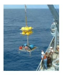
Researchers recovered fluids from beneath the seafloor using specialized deepsea sampling platforms, shown above being deployed from a research vessel and below on-board the ship with UCSC ocean scientist Matt McCarthy.
