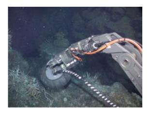
A robotic arm from the ROV Jason II deployed sampling equipment on the seafloor. All photos courtesy of M. McCarthy.
