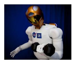
The dexterity and strength developed for Robonaut 2 (R2) enables the robot to complete complex tasks, including lifting and holding a 20 lb. weight, far more than most humanoid robots.
