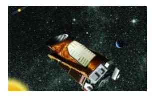
On Dec. 22, 2010, Kepler experienced a safe mode event. A safe mode is a self-protective measure that the spacecraft takes when something unexpected occurs. During safe mode, the spacecraft points the solar panels directly at the sun and begins to slowly rotate about a sun-aligned axis. This safe mode orientation provides the vehicle with the maximum power, and limits the buildup of momentum from the solar wind.
