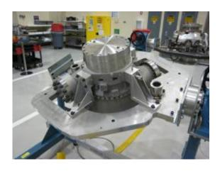
The turbomachinery assemblies for the first development J-2X engine off the production line. Credit: Pratt & Whitney Rocketdyne
