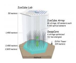
The IceCube neutrino observatory is designed so that 5,160 optical sensors view a cubic kilometer of clear South Polar ice.
