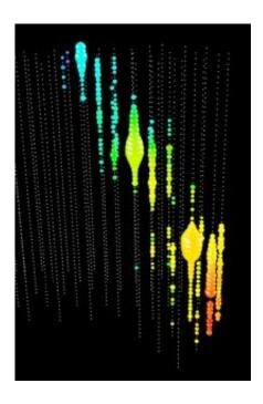
A simulated track of a high-energy neutrino moving upward through IceCube. The circles represent DOMs, and their size represents the amount of light they detect from Cherenkov radiation. Warmer colors are earlier detections.
