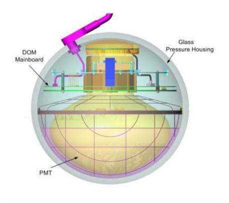
Schematic drawing of a Digital Optical Module (DOM).
