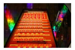
IBM has unveiled a new chip technology, called CMOS Integrated Silicon Nanophotonics chip technology, which enables a 10X improvement in integration density and produces smaller, faster and more power-efficient chips than is possible with conventional technologies. Image courtesy of IBM Research
