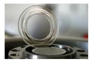
The finished lens array is at a slant behind the lower die set of the hot embossing equipment. (© Fraunhofer IWU)
