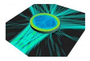
The new microlaser uses an elliptical resonator with a wavelength-sized notch (seen at top right) on the boundary to create unidirectional rays (bottom left). Credit: Courtesy of the laboratory of Federico Capasso, Harvard School of Engineering and Applied Sciences (SEAS)
