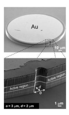
Upper panel: This is a scanning electron microscope image of the notched elliptical resonator with a minor radius  $X=80~\mu m$ , a major radius  $Y=96~\mu m$  and notch dimensions o = 3  $\mu m$ , and d = 2  $\mu m$ . Lower panel: Zoom-in view of the device showing the smooth sidewall of the laser cavity. The two white dashed lines indicate the boundaries of the active region. Credit: Courtesy of the laboratory of Federico Cappaso, Harvard School of Engineering and Applied Sciences (SEAS)
