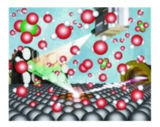
A beam of specially-tuned X-rays scatters off a platinum atom and into a detector, unaffected by the surrounding perchloric acid solution. (Image by Daniel Friebel.)
