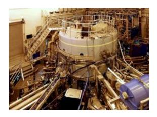
Alcator C-Mod, shown here, is the most powerful university-based fusion device in the world. Recent findings there could help point the way to power-producing fusion reactors. Image: Plasma Science and Fusion Center
