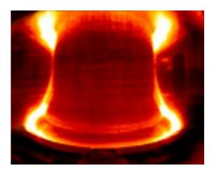
Photo of the interior of Alcator C-Mod during a test run shows the glowing hot plasma, which can reach more than 55 million degrees Celsius. Image: Plasma Science and Fusion Center
